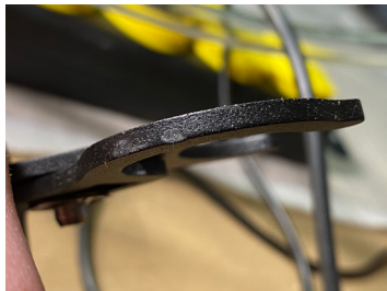
Worn down finish from the metal rod
