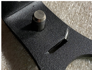
Worn down finish and material on the underside of wall mount from the locking spring
