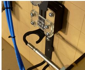
2. Force open by pushing on the locking arm when locked.
