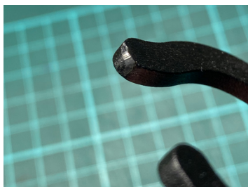
Worn down finish and material from the metal rod
