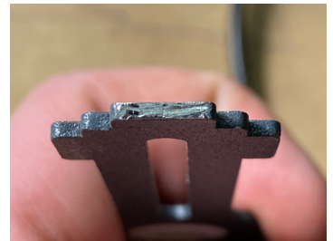
Worn down tip of key from the rotating locking spring
